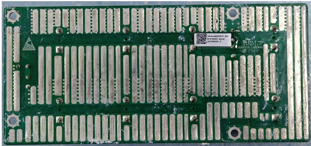
Figure 11 Trace side of BUS. capacitor board
