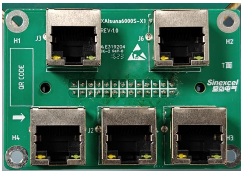
Figure 18 Top of Communication interface board
